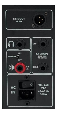
11) FX LOOPS - The FX loops send the signal from the amp post-EQ and return it pre-reverb. The jack is a Tip/Ring/Sleeve type, where the ring is the send and the tip is the return. To use the FX loop you will need a send/return Y-cable, which can be purchased from us or most any music store.
